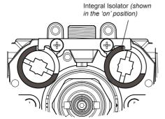
12. Align the slots in the 'black' knob retainer with the lugs on the 'white' hub top and secure the backplate to the mixing valve with the two backplate screws.
