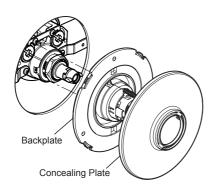
Using a 10 mm hexagonal key turn the integral isolators 90° anti-clockwise to shut off the hot and cold water supplies.
