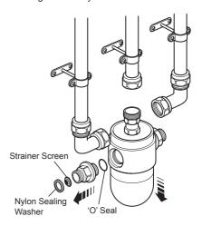
The non return valve cartridge and/or strainer screens can be cleaned or replaced as necessary.
