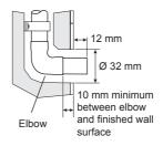
For falling supplies: Mark the pipe positions on the ceiling and set the 33 mm centres from the finished wall.
